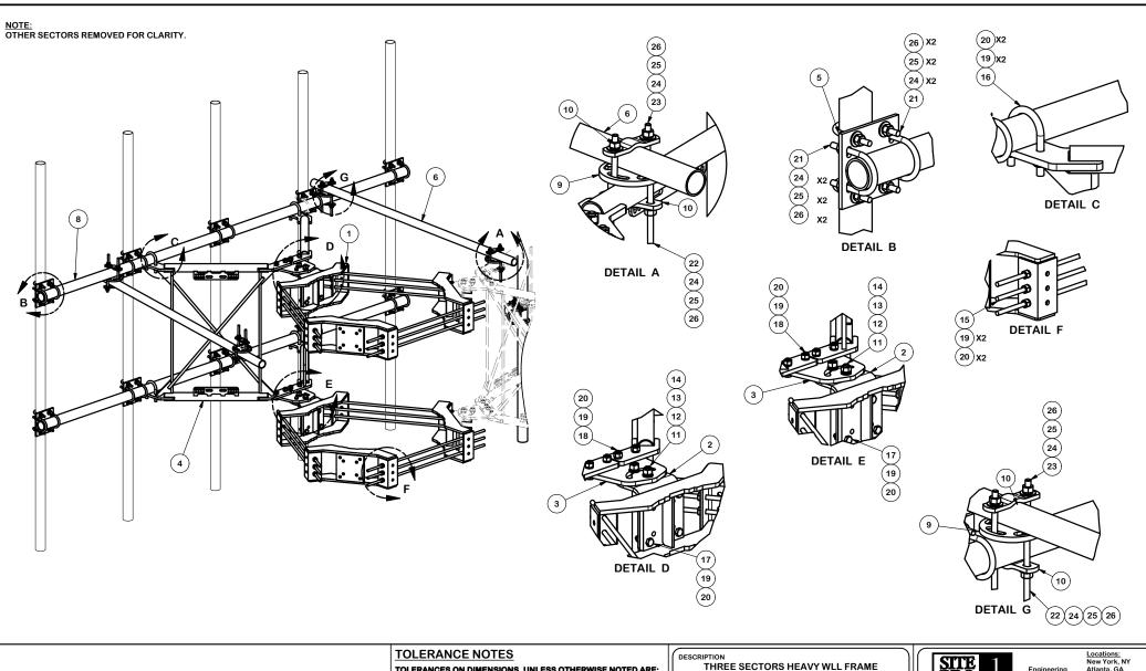
TOLERANCES ON DIMENSIONS, UNLESS OTHERWISE NOTED ARE: SAWED, SHEARED AND GAS CUT EDGES (\$ 0.030") ORILLED AND GAS CUT HOLES (\$ 0.030") - NO CONING OF HOLES LASER CUT EDGES AND HOLES (\$ 0.010") - NO CONING OF HOLES BENDS ARE ± 1/2 DEGREE
